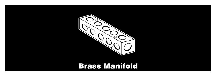
Parker's Brass Manifold provides a convenient junction for the hook-up of multi-branch distribution lines. Porting is easy with five 1/8" and five 1/4" side ports. Two 3/8" inlet ports allow for maximum flow. Universal dual sided 7/32" mounting holes allow for easy manifold attachment.
