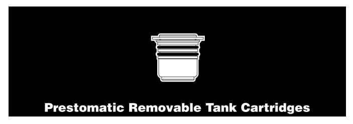
Leakage and assembly problems encountered with the use of pipe threaded fittings in out-of-round internal threads that are commonly found in air tank spuds prompted the development of the Prestomatic<sup>†</sup> Removal Tank Cartridge. This threadless cartridge is retained in the spud by a standard retaining ring, and the double Buna-N (Nitrile) oring seal virtually guarantees leak free performance.
