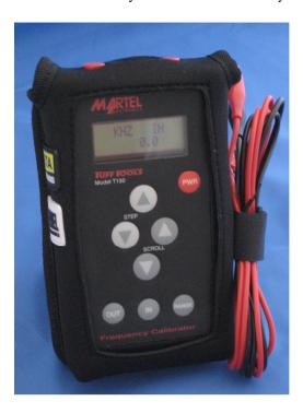
Operation of this calibrator is made easy through the use of a sealed membrane keypad with simple controls. The outputs are set through the use of step and ramp keys which allow both large and small output changes to be made with ease.
