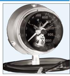
Indicating accuracy of Ashcroft Duragauge, above 300 psi with contact: Pointer not carrying contact – 1.0%; Pointer carrying contact – 1.5%. For ranges below 30 psi, add an additional ½% to indicating accuracies.
