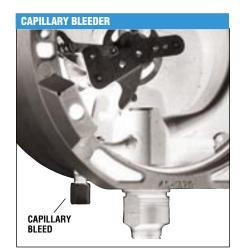
internals of the bourdon tube. It may be used as a pressure testing tap for gauge inspection without removing the gauge from service. Capillary bleeders are available in bottom connected gauges only. The capillary bleeder is available in 300 Series stainless steel and limited to 41/2" 1379(S)S case with 316 stainless steel system. Capillary bleeders are available to 1000 psi.
