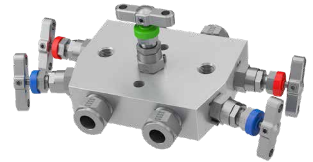
Example shown: 5-valve remote/line mount manifold featuring the Parker A-LOK® Superior Advantage inverted integral tube fitting connections for the impulse line and NPT ported connections for the vent/drain.
