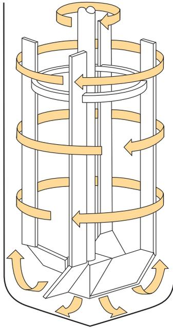
The Elongated Paddle impeller provides a combination of axial upward and radial fluid flow. It, like the Anchor and Helical Impellers, operates in close proximity to the vessel wall.
