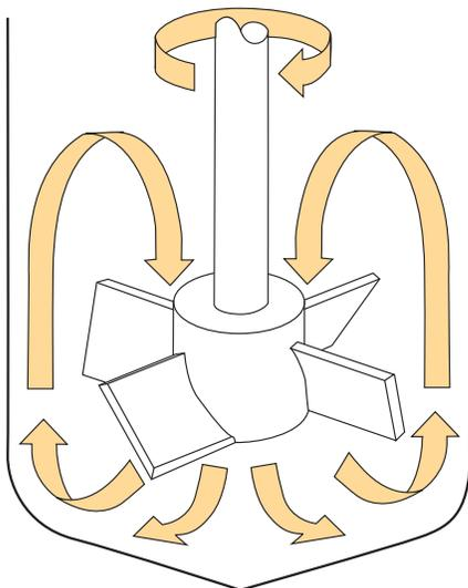
Sometimes termed an “axial flow impeller”, the Pitched Blade Turbine is especially suited for high speed liquid/solid applications where tank baffles may be impractical. Direction of fluid flow can be up or down depending on the pitch. The pitch angle can vary between 0° and 90° from the vertical.
