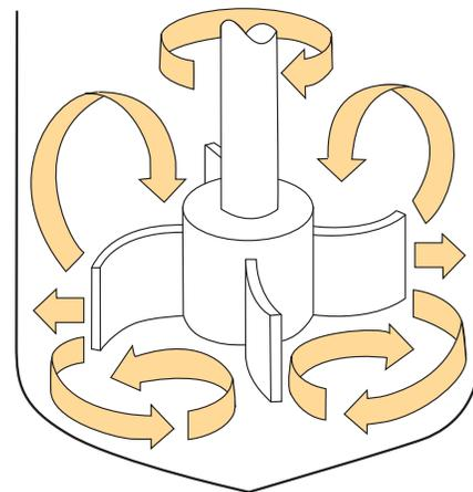
Often referred to as a “backswept turbine”, this impeller can be used in very viscous mixtures where power consumption can be of concern or in liquid/friable solid applications.\* It provides reduced shear and a radial flow pattern. **\*Vessel baffling may be required for optimum performance.**
