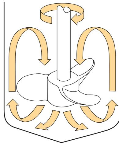
The Marine Propeller is an axial flow impeller generally pitched for downward pumping action, however, upward pumping is also available. This impeller provides a high, uniform discharge and therefore is best suited for low viscosity liquid blending applications.
