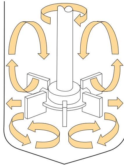
Formerly known as the “Rushton Turbine”, this impeller, like the “AE Dispersimax™ Turbine”, is suited for gas/liquid applications requiring fairly high shear at high speeds.\* The impeller also promotes radial fluid flow. **\*Vessel baffling may be required for optimum performance.**
