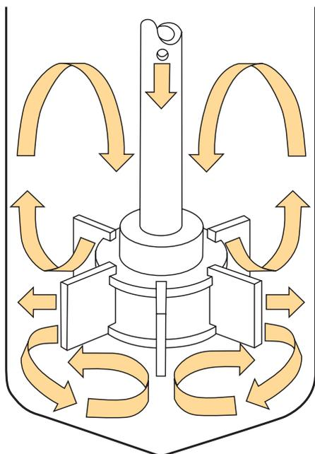
Parker Autoclave Engineers' patented Dispersimax™ Turbine type impeller is well suited for gas/liquid reactions. It provides high speed radial flow stirring, while drawing head space gas down a hollow shaft and dispersing the gas through the impeller ports, for effective entrainment of the gas into the liquid. This is generally for low viscosity applications.\*
