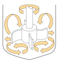
Often referred to as a "backswept turbine", this impeller can be used in very viscous mixtures where power consumption can be of concern or in liquid/friable solid applications.\* It provides reduced shear and a radial flow pattern.\*Vessel baffling may be required for optimum performance.
