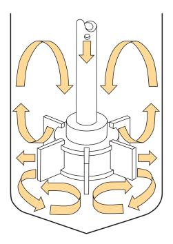
Parker Autoclave Engineers' patented Dispersimax<sup>™</sup> Turbine type impeller is well suited for gas/liquid reactions. It provides high speed radial flow stirring, while drawing head space gas down a hollow shaft and dispersing the gas through the impeller ports, for effective entrainment of the gas into the liquid. This is generally for low viscosity applications.\*
