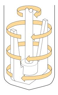
Best suited for high viscosity fluids (5,000-50,000 cp). This impeller provides radial flow and improved heat transfer at relatively low speeds. It generally provides minimal radial clearance between it and the vessel wall. Anchor impellers can be provided with wipers and/or cross arm support.
