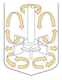
Formerly known as the "Rushton Turbine", this impeller, like the "AE Dispersimax<sup>™</sup> Turbine", is suited for gas/liquid applications requiring fairly high shear at high speeds.\* The impeller also promotes radial fluid flow. \*Vessel baffling may be required for optimum performance.
