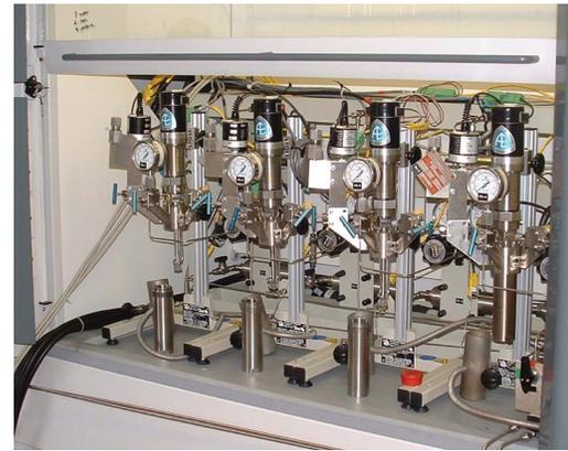
Parker Autoclave Engineers MagneDrive® is a magnetically coupled, packless rotary impeller system designed to provide continuous high speed mixing without leakage or contamination. Utilizing the rare earth magnetic technology which Parker Autoclave Engineers developed and was the first to market in 1958, the packless MagneDrive® eliminates the process contamination, lubrication, packing friction, shaft cooling and maintenance problems common with other forms of mixing.
